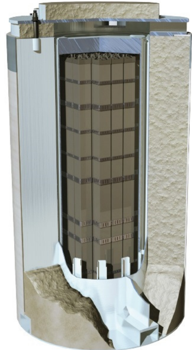
Cutaway of spent fuel storage cask shows spent fuel assemblies surrounded by steel and thick concrete shielding.
