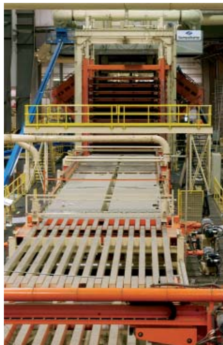
The press with the press loader
