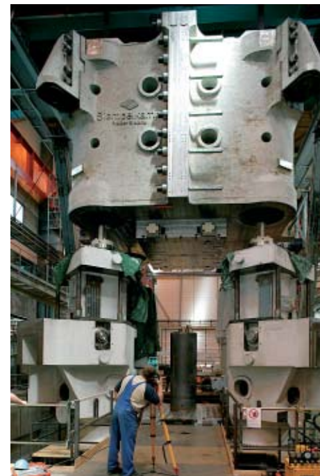
The upper cross-beam will be lowered over the tie-rods
