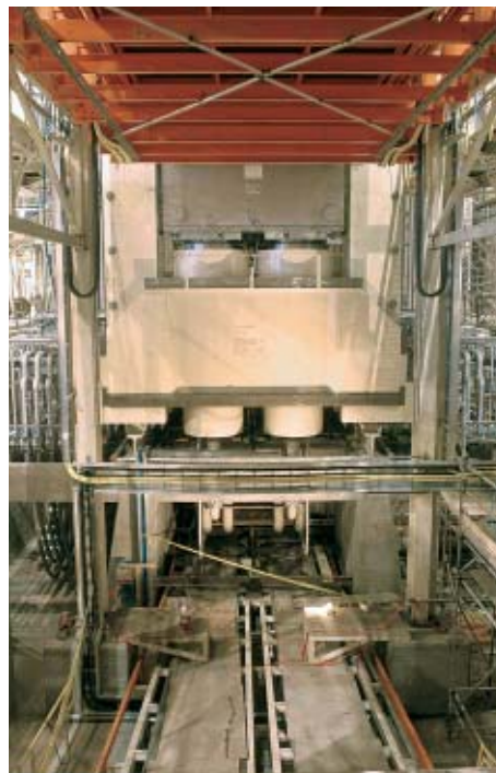
The press pit with the belt conveyor for the screens
