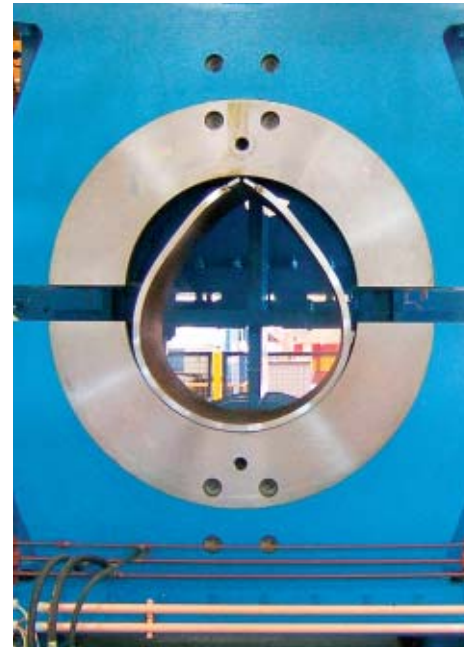
... finally the O-forming for the closing of the pipe
