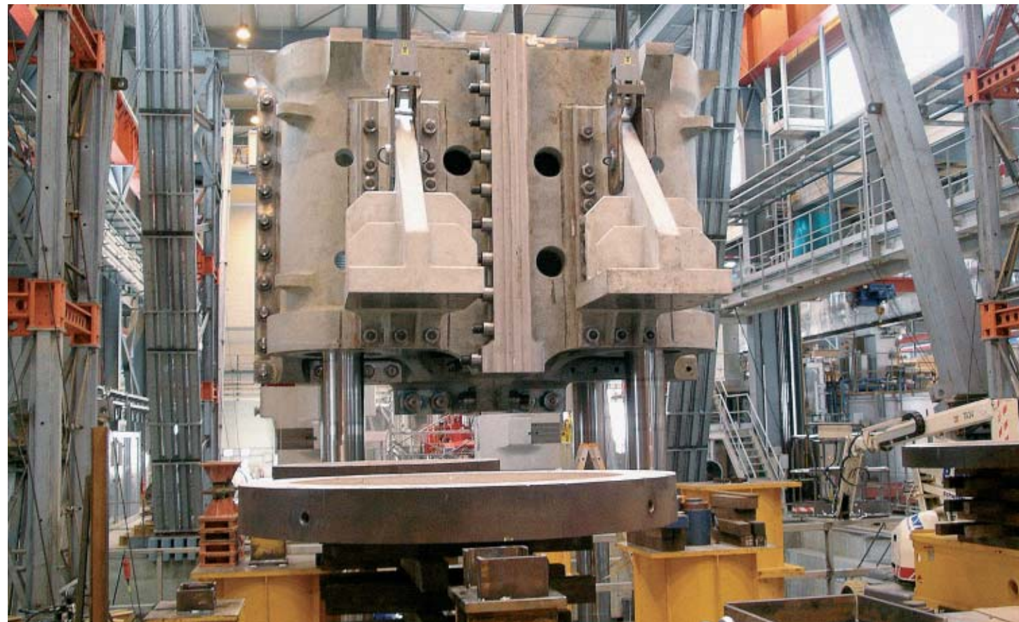
The lower cross-beam, 1,360 t, is hanging on the strandjack
