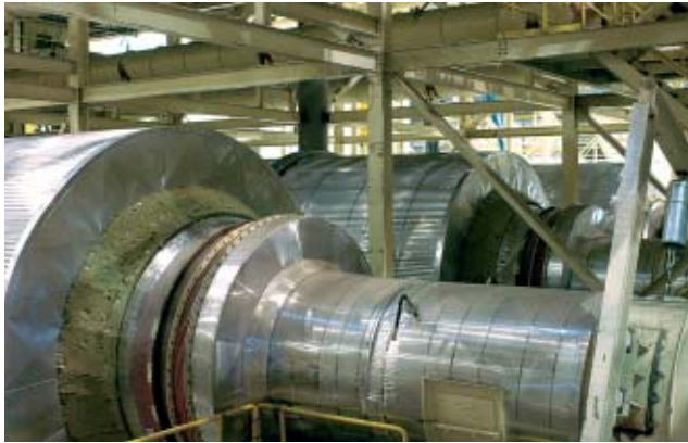
Three drum dryers side by side: even if one aggregate fails or needs to be maintained the plant can continue running at full capacity
