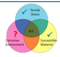
2/3 of the requirement for SCC are present in welded stainless steel canisters
