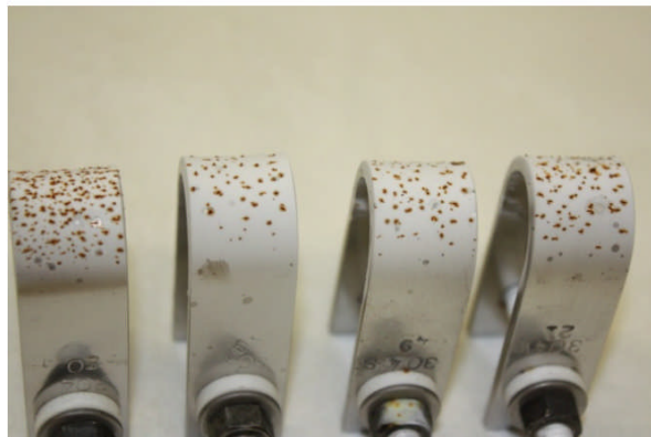
Figure 3. Surface Corrosion Deposits on CISCC U-Bend Specimens
