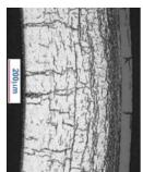
Figure 1 significant radial cracks in fuel cladding
