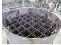
37 fuel assembly thin-wall canister
