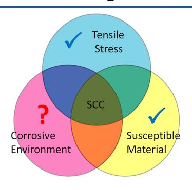
2/3 of the requirements for SCC are present in welded stainless steel canisters
