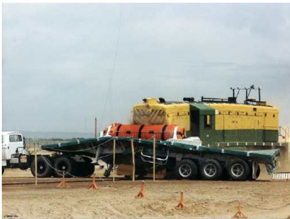
Figure 5. Spent-Fuel Crash Test
