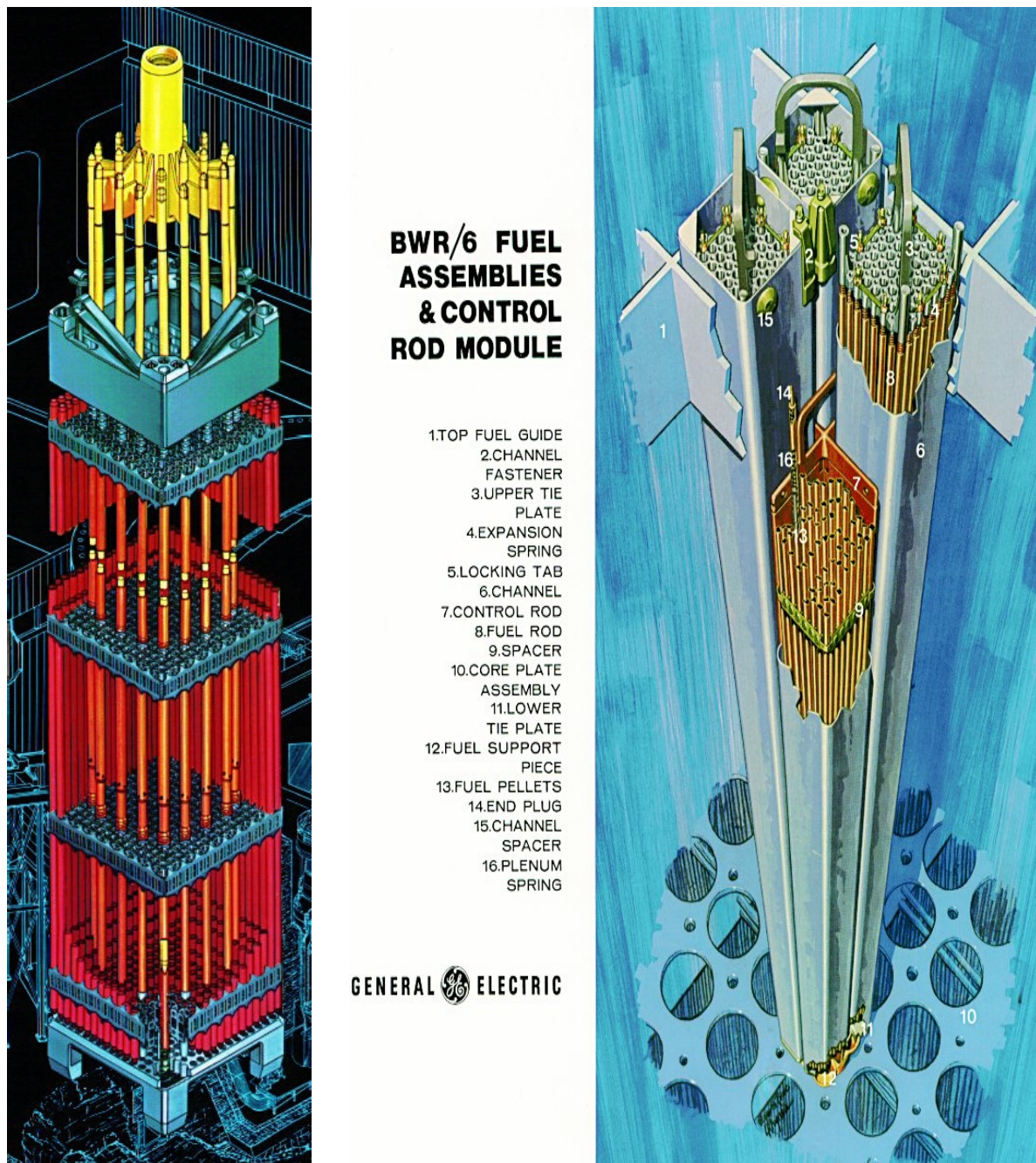
Figure 18. Typical PWR and BWR Fuel Assemblies
