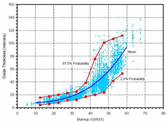
Figure 20. Cladding Outer Surface Oxide Layer Thickness versus Rod Average Burnup
