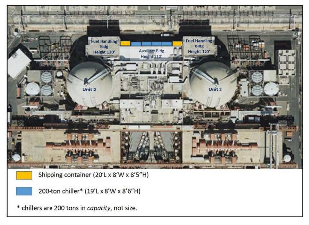
**Above**: Configuration of the shipping containers and chillers between the Units 2 and 3 fuel handling buildings (Note: shipping container and chiller representations not to scale; the area that will be occupied is less than half the space shown in this figure)
