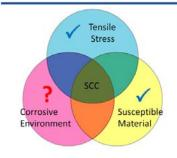
2/3 of the requirements • for SCC are present in welded stainless steel canisters
